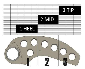
You can start adjusting from the image below. Don't be overly concerned about exat weight placement at this time, it's only starting point. Your machine should run in most cases 7200-7400rpm.
