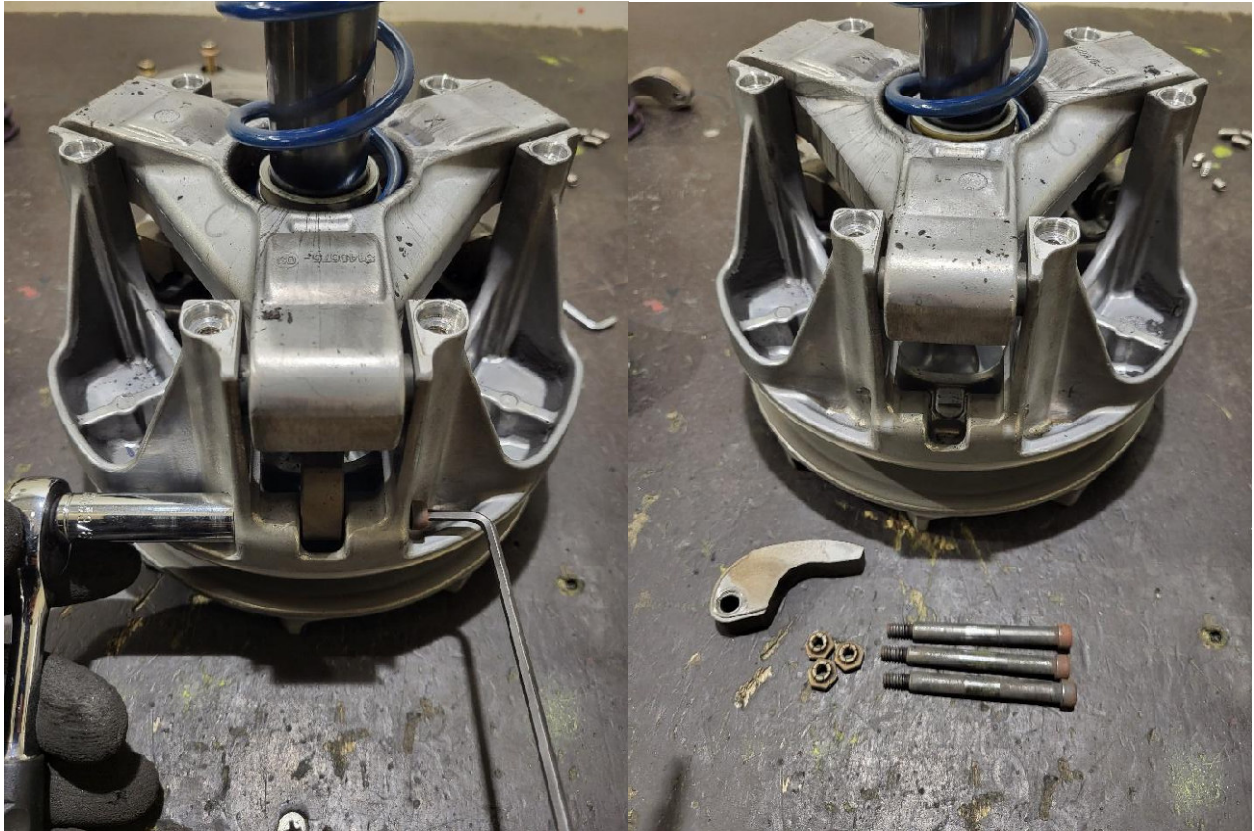
14. Remove primary clutch weight pins and original weight arms.
