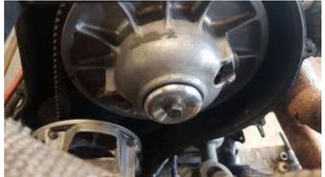
When tightening the upper variator, tighten the central screw (15 mm ring spanner or ratchet) with 65 NM (originally we use blue screw lock)
