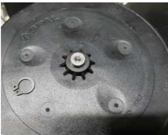
Align the fan and attach it to the secure clip. Make sure that the fan wheel rotates freely and without contact.
